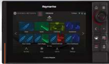
Raymarine AXIOM PRO 9 S chart plotter with HybridTouch multifunction display at helm station, stb
